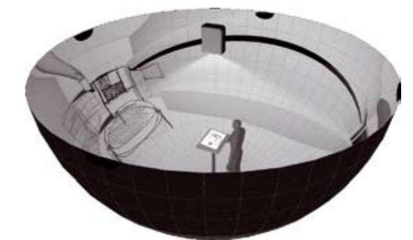
Figure 3: iDVR system: Panoscope with pivoting digital pad.
